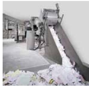
**AUTO-FEED™ Systems** Allegheny's revolutionary AUTO-FEED™ Systems greatly increase your shredding capacity while significantly reducing your labor costs. These systems utilize a high capacity Primary Conveyor (in-floor or above-ground) coupled with a variable-speed Metering Conveyor,
