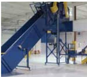
**Conveyors** Allegheny offers Sorting Conveyors, which allow several operators to separate materials by grade and type prior to shredding to maximize the value of your recycled paper. We also offer Primary Conveyors (in-floor or above-ground), Metering Conveyors (see AUTO-FEED™ Systems
